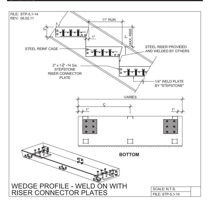
PRECAST CONCRETE TREADS AND LANDINGS SHOWN ON PLANS SHALL BE FROM THE LONG SPAN "STEPTREAD" SYSTEM BY "STEPSTONE, INC." OF GARDENA, CA FOR STEEL CONSTRUCTION. THE MANUFACTURER IS TO SUPPLY ALL PRECAST CONCRETE "STEPTREAD" SYSTEM PARTS, FEATURING BOTTOM WELD PLATES FOR WELD-ON CONNECTIONS. ALL REINFORCING AND CONNECTION PLATES WILL BE ZINC PLATED. ONLY ITEMS NOTED AS BY "STEPSTONE, INC." WILL BE FURNISHED BY "STEPSTONE, INC." SUCH ITEMS ARE TO BE INSTALLED BY OTHERS. Page 46-LS
